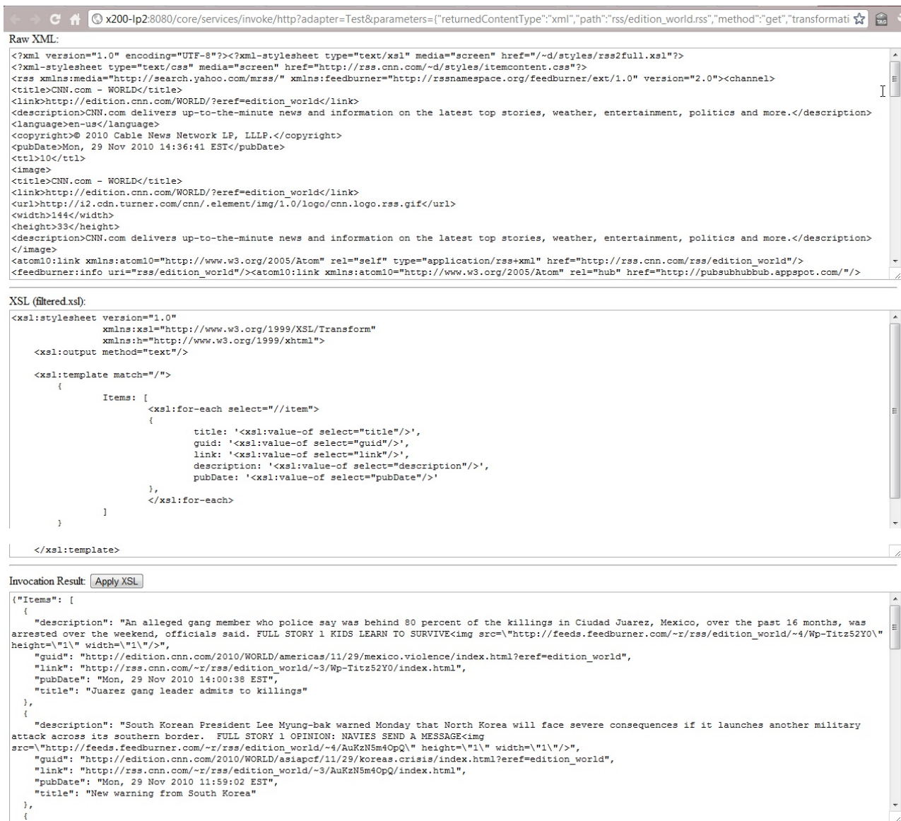
Figure 8-48. Browser window, showing retrieved data in XML and JSON format.
