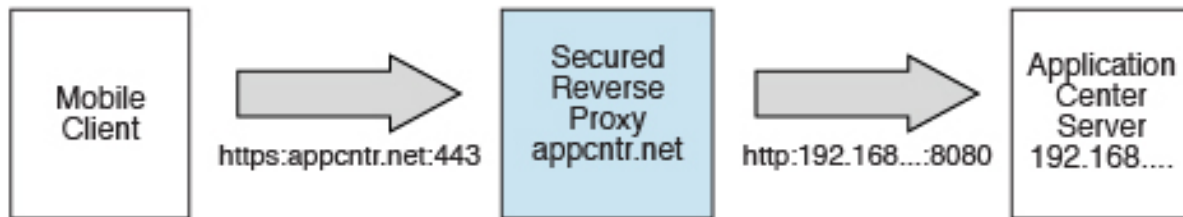
Figure 6-25. Configuration with secured reverse proxy
