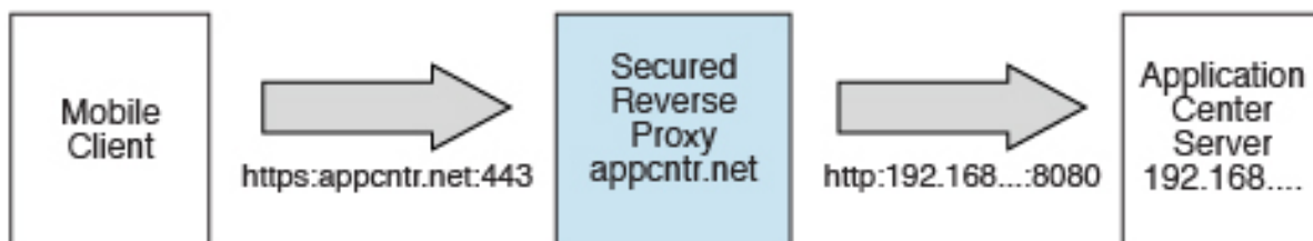
Figure 6-17. Configuration with secured reverse proxy
