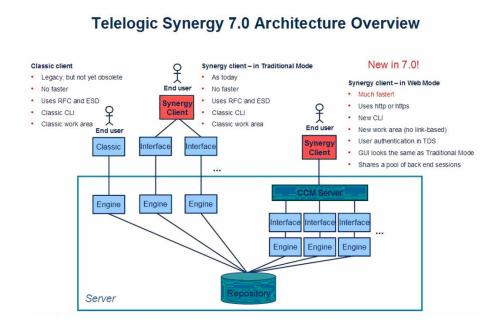
Web mode clients connect to a Telelogic Synergy Web server via HTTP. The Telelogic Synergy server manages a pool of back-end sessions, which all run on the server system.
