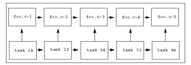
The foo.c file has five versions. Each version is associated with a different task. (The task number associated with each version is shown below the object version.)
