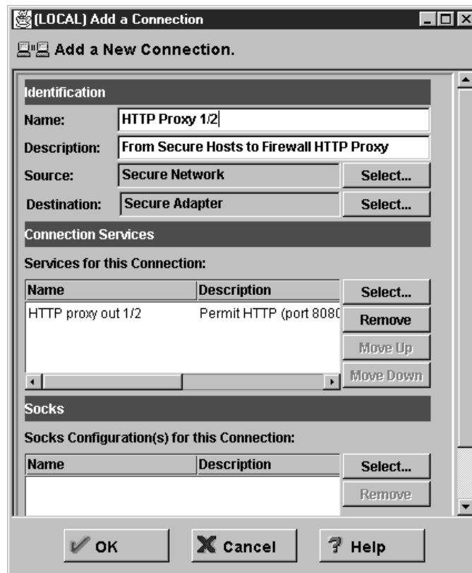
Figure 278. HTTP Proxy Connection on Secure Network
