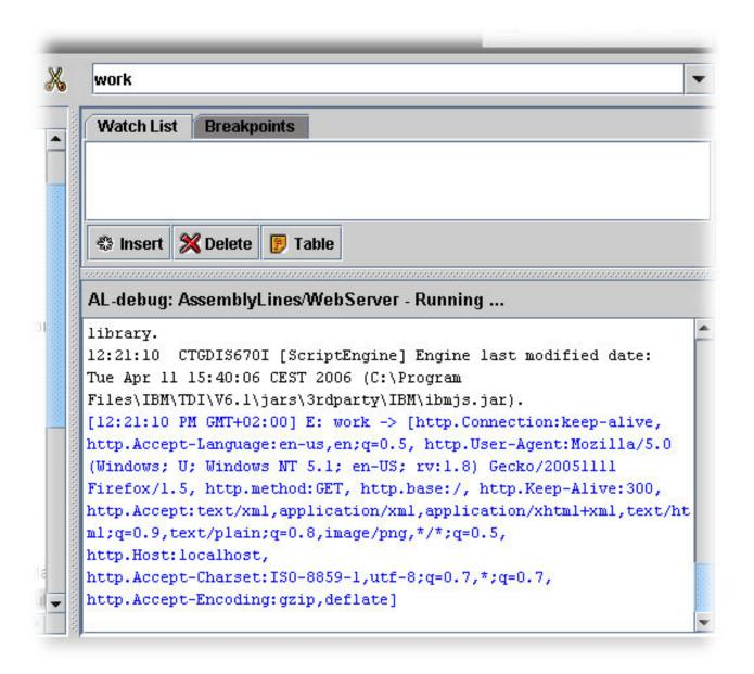
Because the output is not easy to read, press Ctrl+A to select "work" and replace it with "task.dumpEntry(work)". When you press Enter this scripted function call actually writes messages to the log, just like it does when run from a script inside your solution, so you should now see an Entry dump in the output window.<sup>21</sup>
