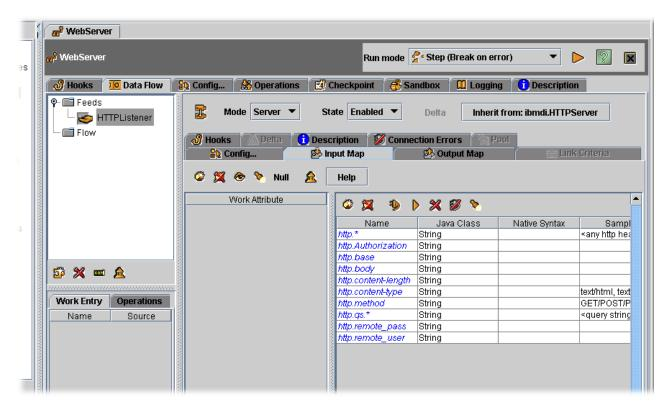
The schema for this Connector is already discovered. Like the other Server Mode Connectors, it has a hard-coded Schema.<sup>19</sup> This is because it's difficult to connect and discover the schema of a client. You have to have one connect to you first. So for convenience, these components show you what to expect.
