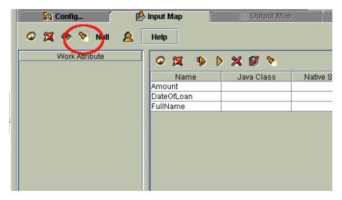
This convenient button makes the Connector connect to its source, do a single *GetNext* on the data set and then examine the returned Entry. The attributes found here are displayed in the Connector Schema list and are ready for mapping. Now although this does not discover all the attributes defined in the schema of the data source (you need to use the **Discover Schema** button found at the top of the Connector Schema list for this) it is enough for you to continue your work.
