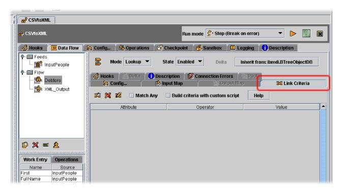
Selecting this tab brings up the Link Criteria display where you can create one or more simple Link Criteria matching rules. These rules are AND'ed together by the Connector to make the system-specific call; or if you select the Match Any check box, then a logical OR is used instead. Since each Connector knows how to translate your Link Criteria to the relevant syntax for the underlying data source, your solution is kept technology-independent.<sup>15</sup>
