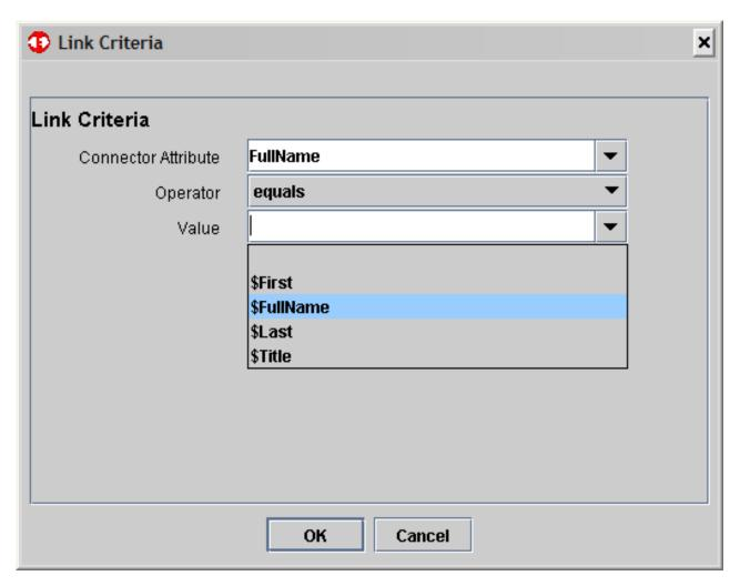
Notice how the **Value** menu only shows you those Attributes that are present in the flow *before* this Connector is reached. Those Attributes brought into the AssemblyLine by the **Debtors** Connector are not available yet, and cannot be used to set up Link Criteria at this point.
