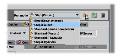
This starts your AssemblyLine just like clicking **Run**, except that your AssemblyLine is running in interactive mode. Instead of the usual log output display, the Debugger window opens instead.
