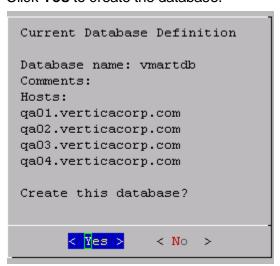
During database creation, Vertica automatically creates a set of node definitions based on the database name and the names of the hosts you selected and returns a success message.
