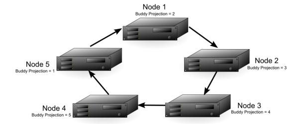
The diagram above shows a 5-node cluster that has a K-safety level of 1. Each of the nodes contains buddy projections for the data stored in the next higher node (node 1 has buddy projections for node 2, node 2 has buddy projections for node 3, etc.). Any of the nodes in the cluster could fail, and the database would still be able to continue running (although with lower performance, since one of the nodes has to handle its own workload and the workload of the failed node).
