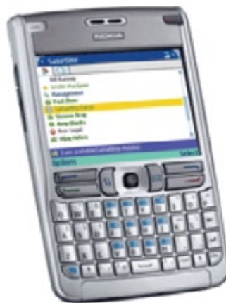
Figure 2. The Lotus Sametime mobile client running on a Nokia E series device
