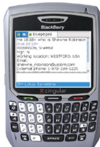
Figure 4. An example of BOT access to a corporate directory from a Lotus Sametime mobile client running on a RIM BlackBerry device
