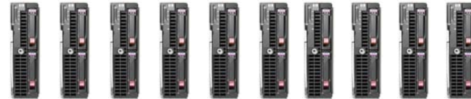
Exchange Mailbox Servers 10 x BL460c G6 (8 core, Xeon E5504 2.00 GHz)
