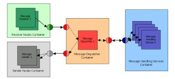
The diagram above presents the simplified high-level architecture of the MHF, detailing receivers, dispatcher, services, and senders within their respective containers.
