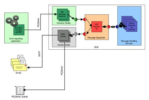
In general, an application that detects an error and has access to the EHF client component can use the component to report the error condition. The following report fields can be set by the error-reporting application through the EHF client:
