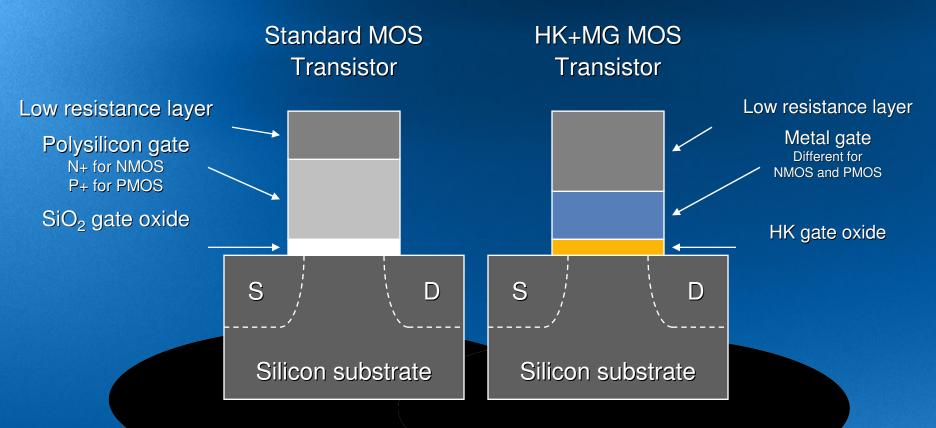
High-k + metal gate transistors provide significant performance increase and leakage reduction, ensuring continuation of Moore's Law
