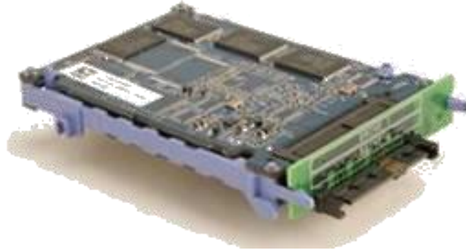
Figure 4 – IBM's Dual-stacked, Solid State Drive Designed for IBM Blades
