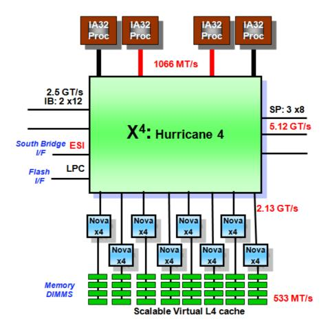
Now each processor has its own channel to the controller, the speed has been increased and each memory set has its own cache.
