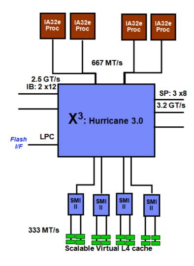
The main part of this diagram shows the number of the channels to the IA32e processors and to the L4 cache. With X3 there was one channel per processor and each pair shared a channel to the controller. With the advent of multi core processors these channels had to provide throughput for either two (dual core) or four (quad core) sets of CPU cycles.
