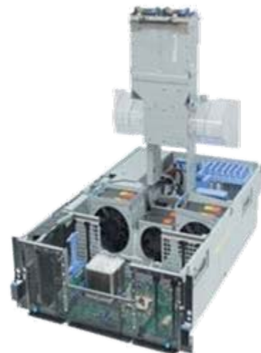
Power off un-used slots, variable fan speed based on ambient temperature
