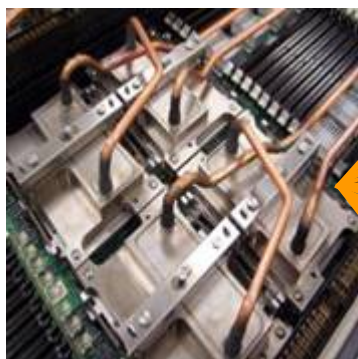
80% heat load to water 40% energy savings via improved cooling and power efficiencies
