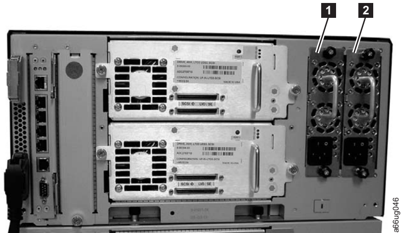
Figure 11-1. Power supplies in a control module
