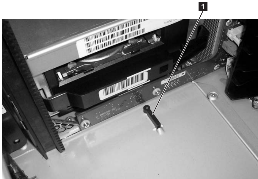
Figure 3-10. Y-axis/Picker Home Sensor Flag
