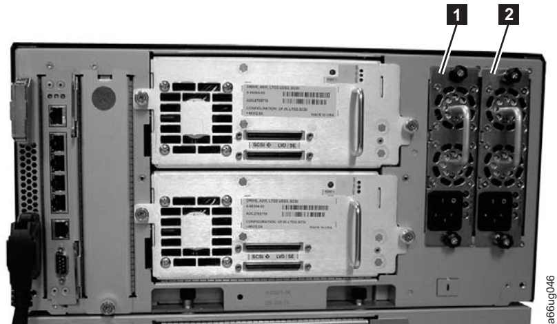
Figure 8-41. Power supplies in a control module
