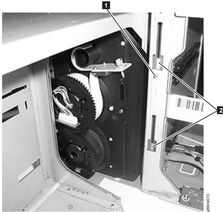
Figure 8-70. Rear gear rack location on chassis
