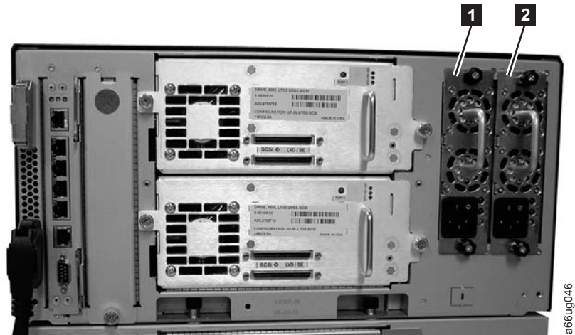
Figure 2-8. Power supply location coordinates
