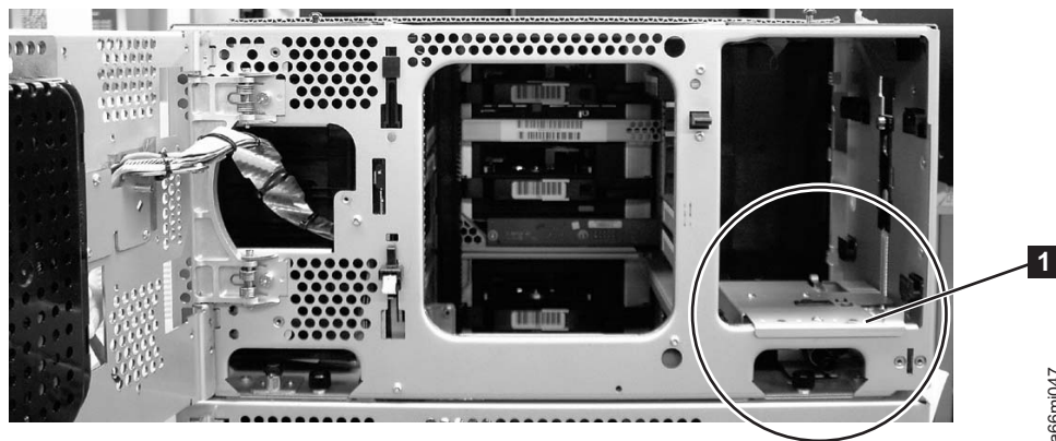
Figure 8-23. I/O Station Lock Assembly installed in library
