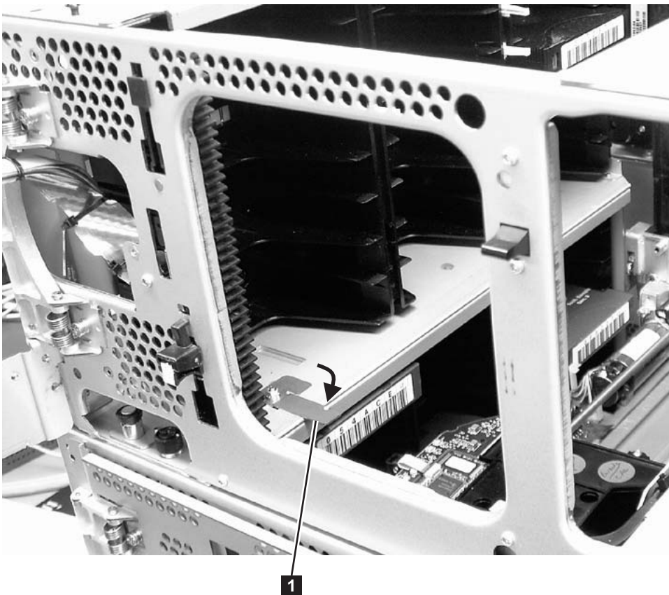
Figure 12-1. Picker locking mechanism
