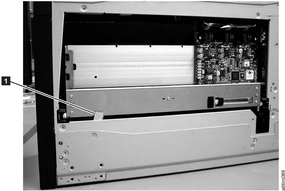
Figure 4-14. Bottom view of picker assembly lock mechanism
