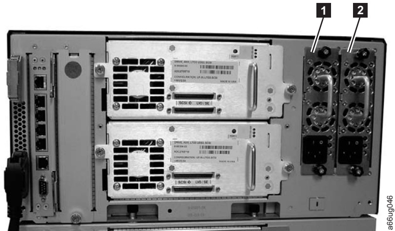
Figure 12-22. Power supplies in a control module
