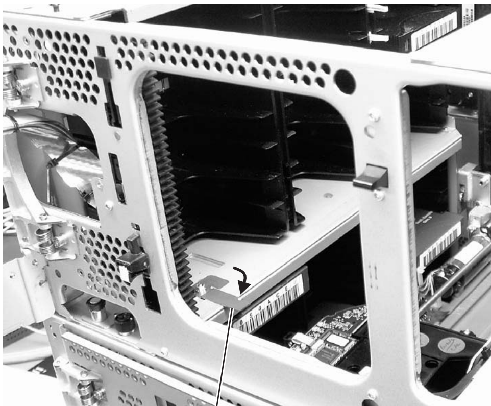
Figure 12-11. Picker assembly locking mechanism
