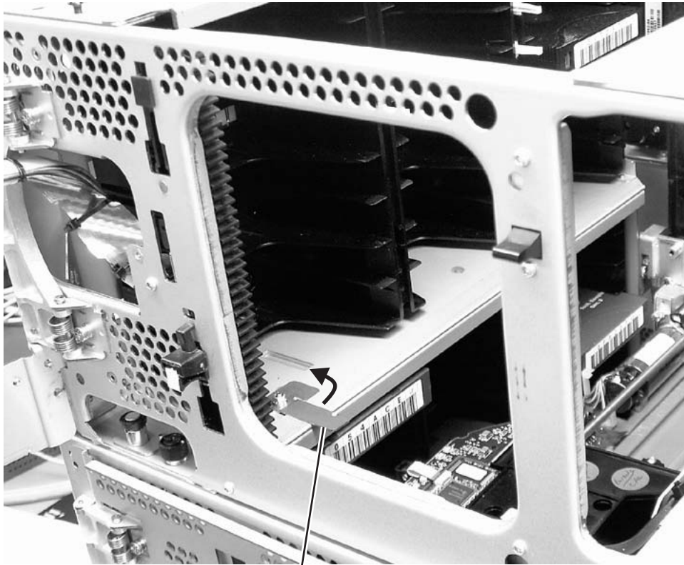
Figure 4-19. Releasing the picker assembly lock mechanism
