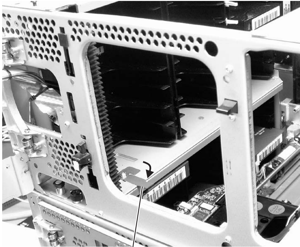
Figure 4-7. Picker locking mechanism
