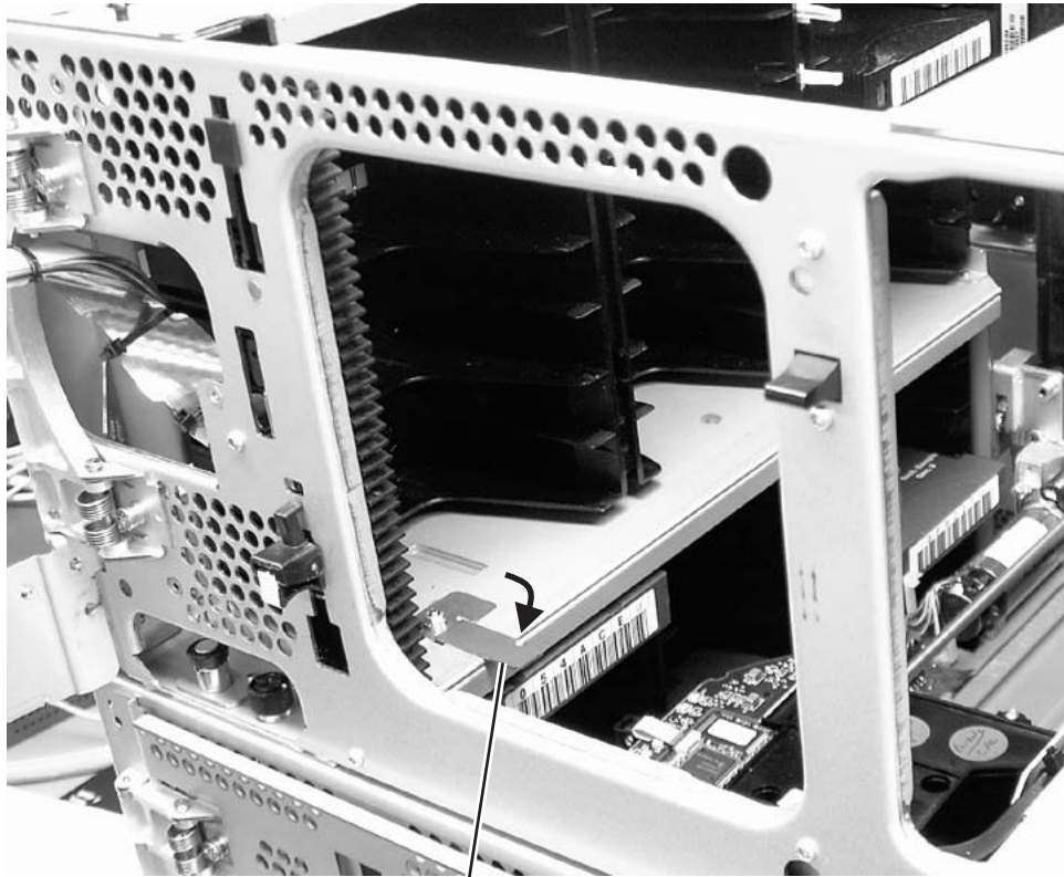
Figure 3-21. Picker assembly lock mechanism
