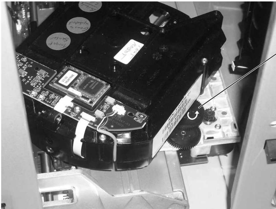
Figure 7-16. Picker rotated for drive gears access
