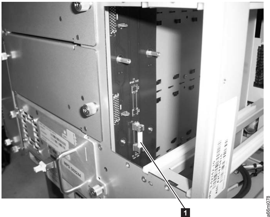
Figure 8-70. Drive power overload fuse
