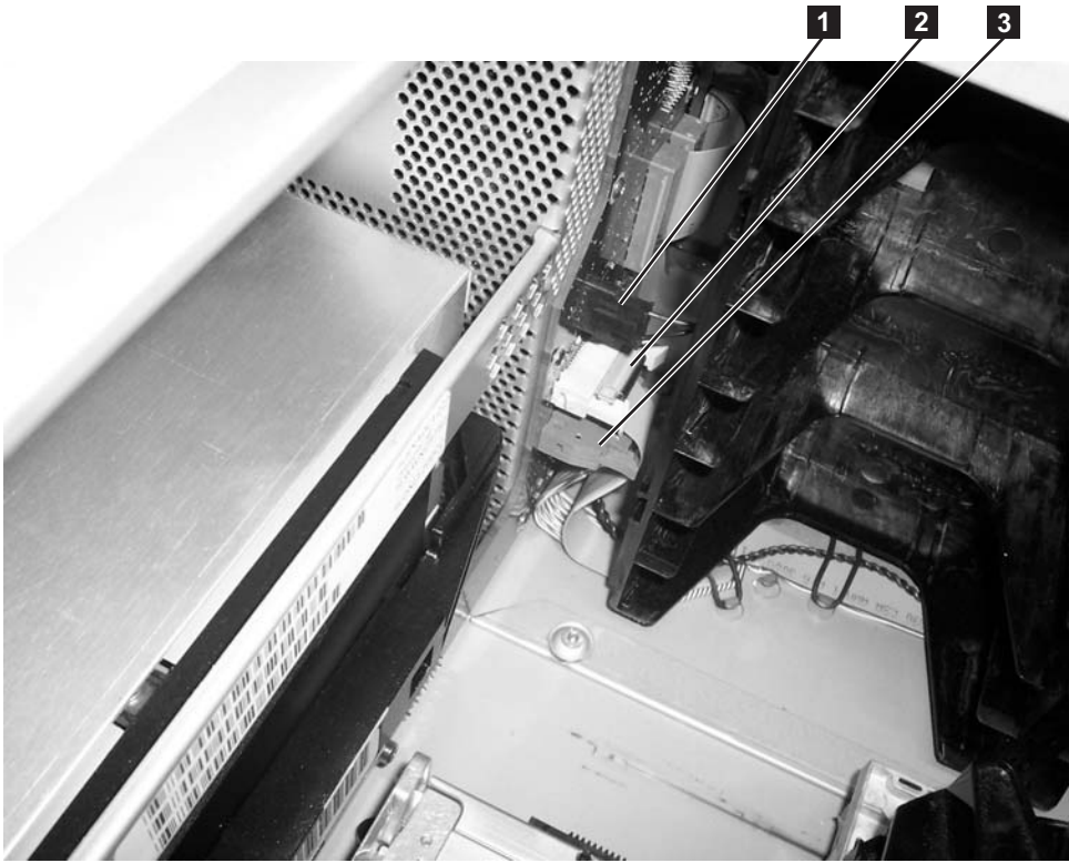
Figure 7-11. Backplane Connect Board connectors (front, top cover removed)
