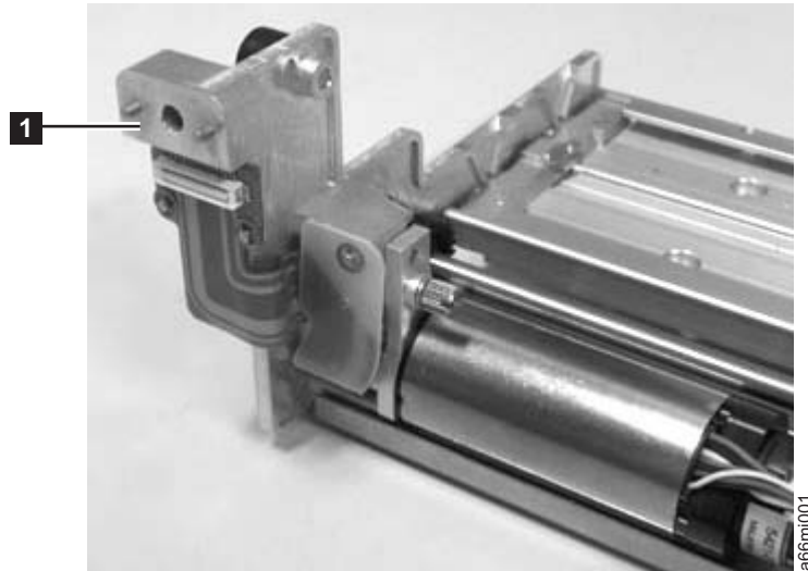
Figure 8-35. Thumbscrew securing Cable Spool
