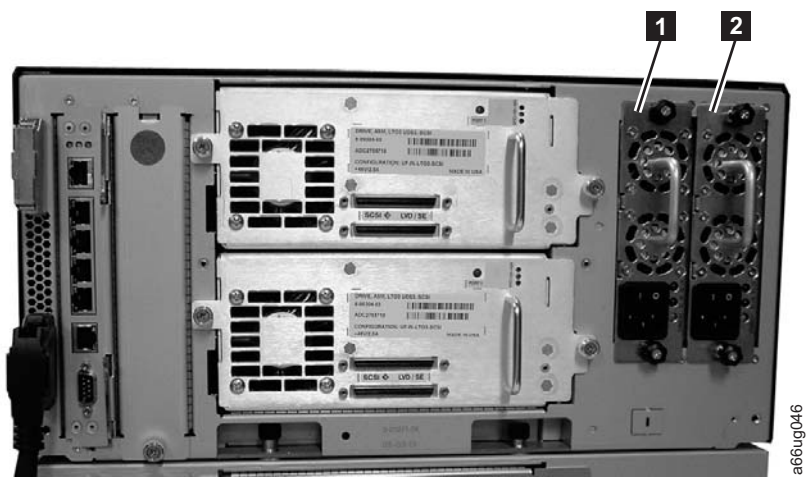
Figure 8-31. Power supplies in a control module
