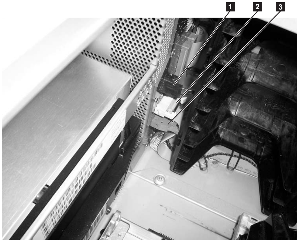
Figure 8-16. Connector between the storage column 4 magazine and Library Control Blade (top cover removed)
