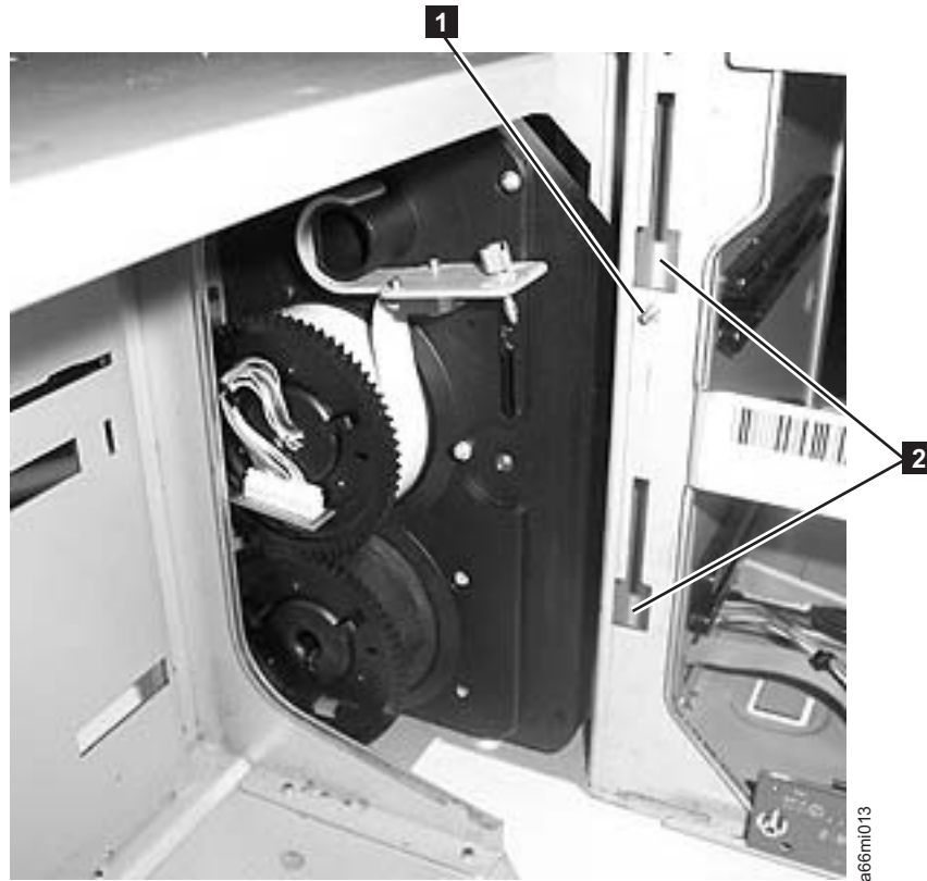
Figure 8-60. Rear gear rack location on chassis
