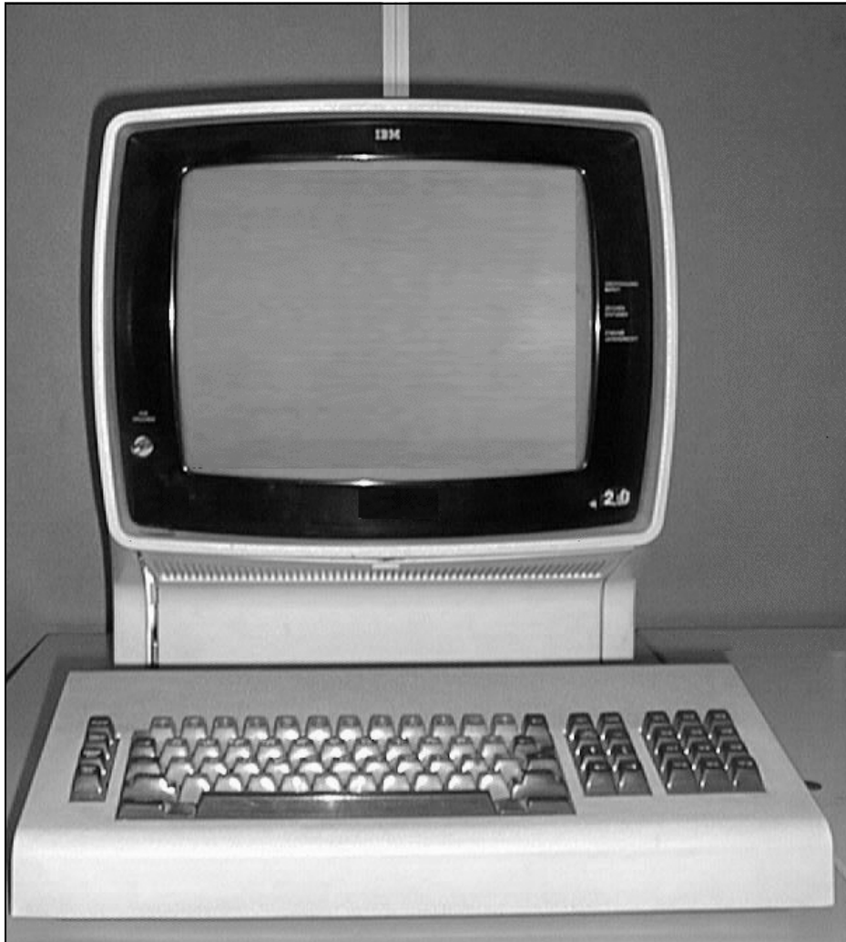
Figure 10-1 IBM 3270 Display Terminal
