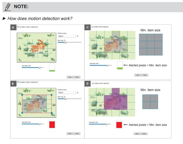
There are two motion detection parameters: Sensitivity and Min. Item Size. As illustrated above, frame A and frame B are two sequential images. Pixel differences between the two frames are detected and highlighted in gray in which the sensitivity setting will take effect. Sensitivity is a value that expresses the sensitivity to moving objects. A higher sensitivity setting allows camera to detect slight movements while a lower sensitivity setting will neglect them.
