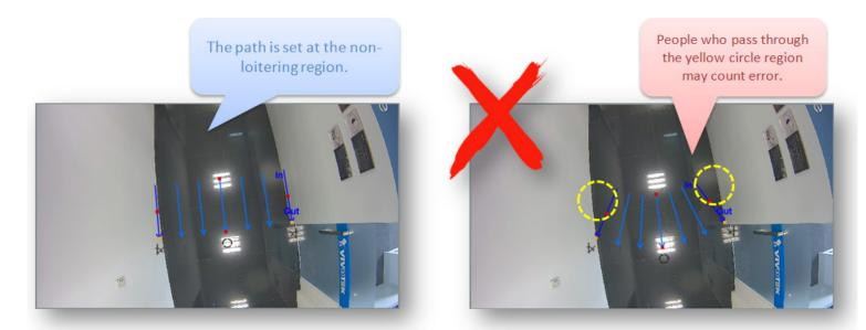
• Set the flow path width according to the aisle that the people's feet will pass through.
