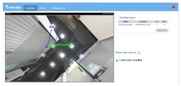
In this common scenario, you may want to count the number of passengers passing this section of a passageway (aisle). It is recommended to adjust the parallel flow path direction and make sure that the flow path arrows are covering the popular walking routes. If the passageway is close to the corner, for example, you could slightly expand the centre angle of the flow path to cover the route of random turns.
