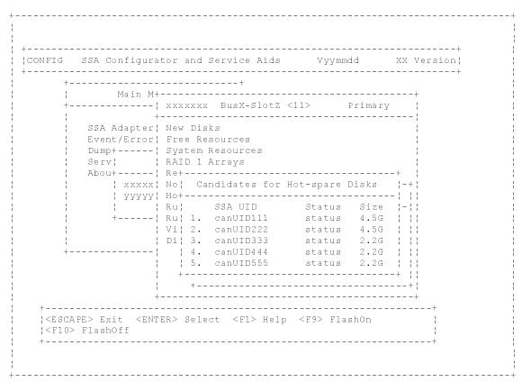
6. Highlight the entry for the disk drive that is to be the hot spare. (You can identify the disk drive by putting the cursor on its Unique ID in this list and pressing F9. This causes a light on the disk drive to flash. Pressing F10 stops the light flashing.) Press Enter to define this disk drive as a hot spare.
