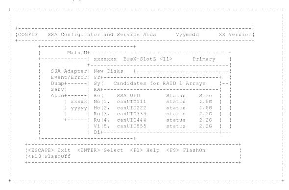
c. Select the disk drive that is to be included in the array. (You can identify the disk drive by highlighting its Unique ID in this list and pressing F9. This causes the Check light on the disk drive to flash. Pressing F10 stops the light flashing.)
