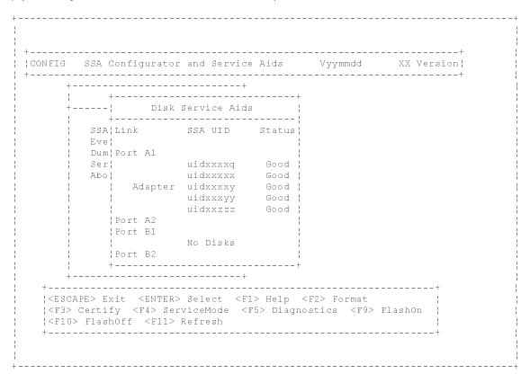
In this example, four disk drives are connected between ports A1 and A2 of this adapter, in a loop, in the order shown, with the SSA adapter in the other system. There are no disks connected to ports B1 and B2.
