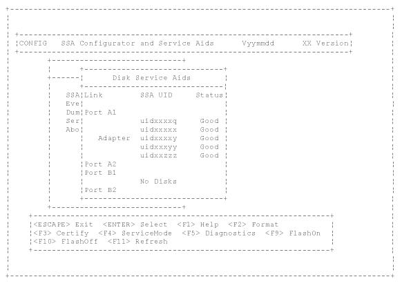
In this example, four disk drives are connected between ports A1 and A2 of this adapter, in a loop, in the order shown, with the SSA adapter in the other system. There are no disks connected to ports B1 and B2.
