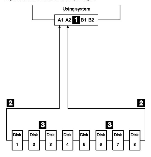
If a disk drive fails, or is turned off, the loop is broken, and one of the data paths to a particular disk drive is no longer available. The disk drives on the remains of the loop continue to work, but an error is reported to the system.
