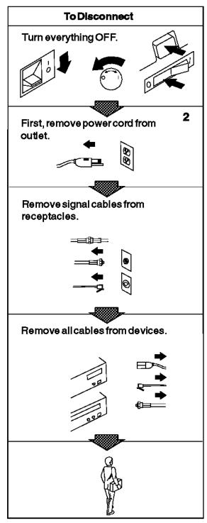
2 In the U.K., by law, the power cord must be disconnected after the telephone line cable
