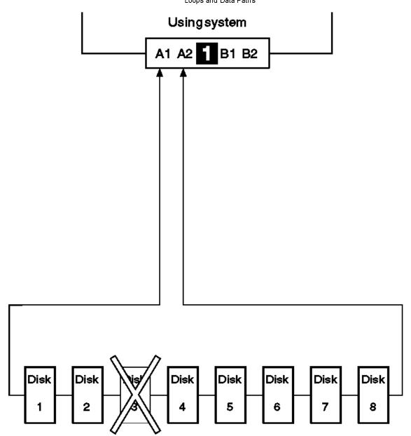
If two or more disk drives are turned off, fail, or are removed from the loop, some disk drives might become isolated from the SSA adapter.
