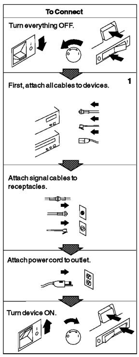
1 In the U.K., by law, the telephone cable must be connected after the power cord
