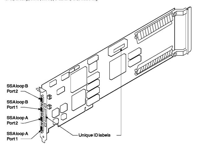
On the adapter card, there is a light next to the pair of SSA connectors (port 1 and port 2) for each SSA loop.
