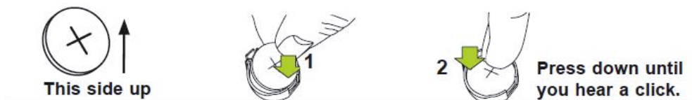
Figure 20. Install the battery
