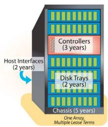
What really doesn't change is the array chassis. One can slide modular components in and out of the chassis pretty much at will. In fact, the array chassis can remain in place and in productive use for many years so long as its modular components can be replaced as needed to either maintain a consent level of reliability or keep pace with technological advancement.
